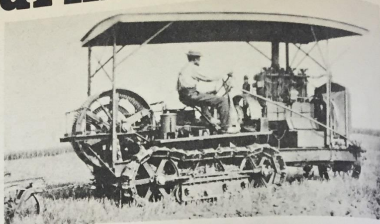
J.C. Ackerman in 1909 using a Holt Caterpillar Tractor to plow. Caterpillar came out to the Ackerman farm to see how efficient this tractor would be in furnishing belt power for a threshing machine. They used the tractor to plow the Ackerman and Eli Staker land.
